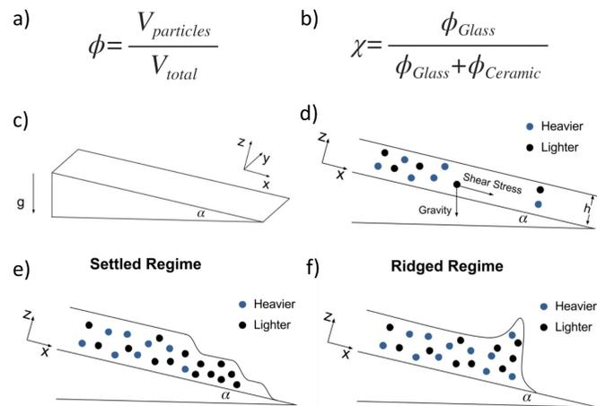
**Figure 1** a) equation describing the total volume fraction  $\Phi$  b) description of volume ratio of beads  $\chi$  c) view of the track with coordinates d) side view of the track with forces e) typical settled regime behavior: heavier particles settle out of the flow, followed by lighter particles, leaving a clear fluid front. f) typical ridged regime behavior: particles migrate to the front of the flow, creating a ridge.
