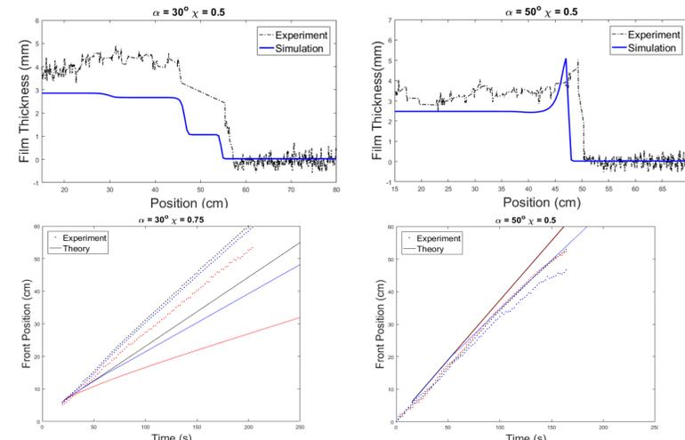
**Figure 2** Experimental results superimposed with simulations generated by mathematical model. Clockwise from top left: height profile of settled regime, height profile of ridged regime, front position of ridged regime, and front position of settled regime.
