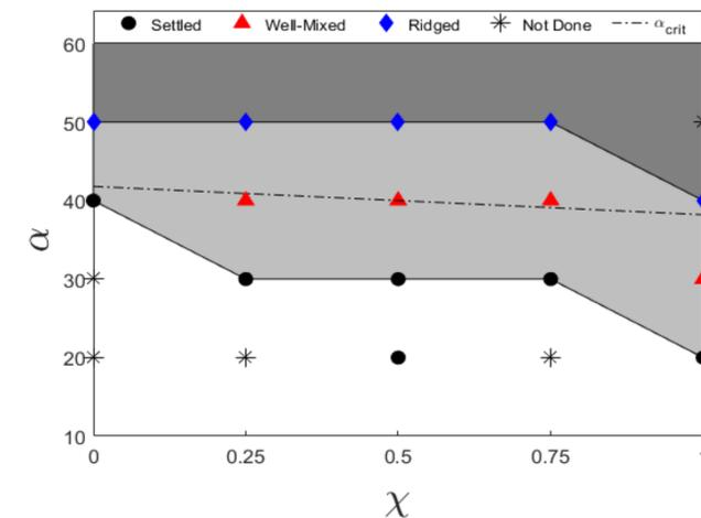
**Figure 4: Phase Diagram** Markers specify experimental trials. Shading indicates the ridged (dark grey), well-mixed (light grey), and settled (white) regimes. The theory suggests that eventually, the boundary between settled and ridged regimes is the dotted line.
